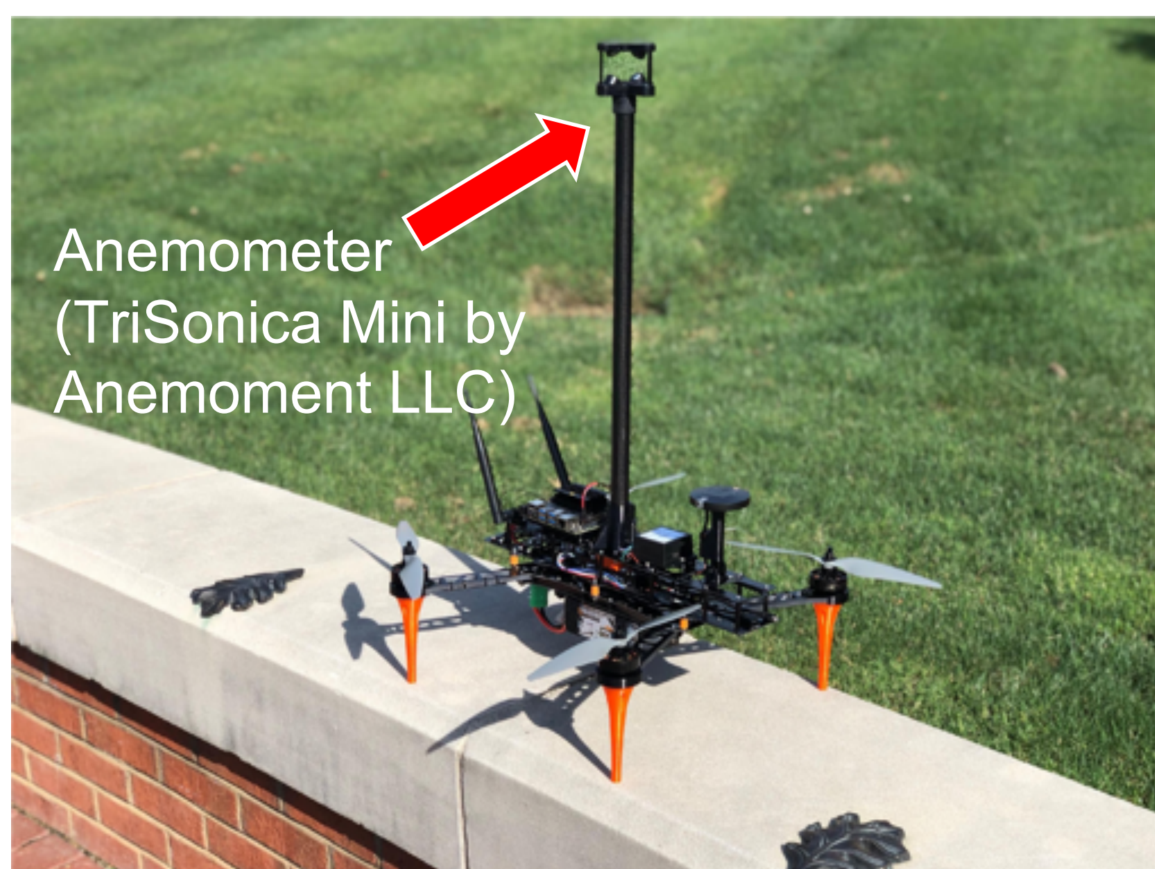
The ARSL drone with anemometer
