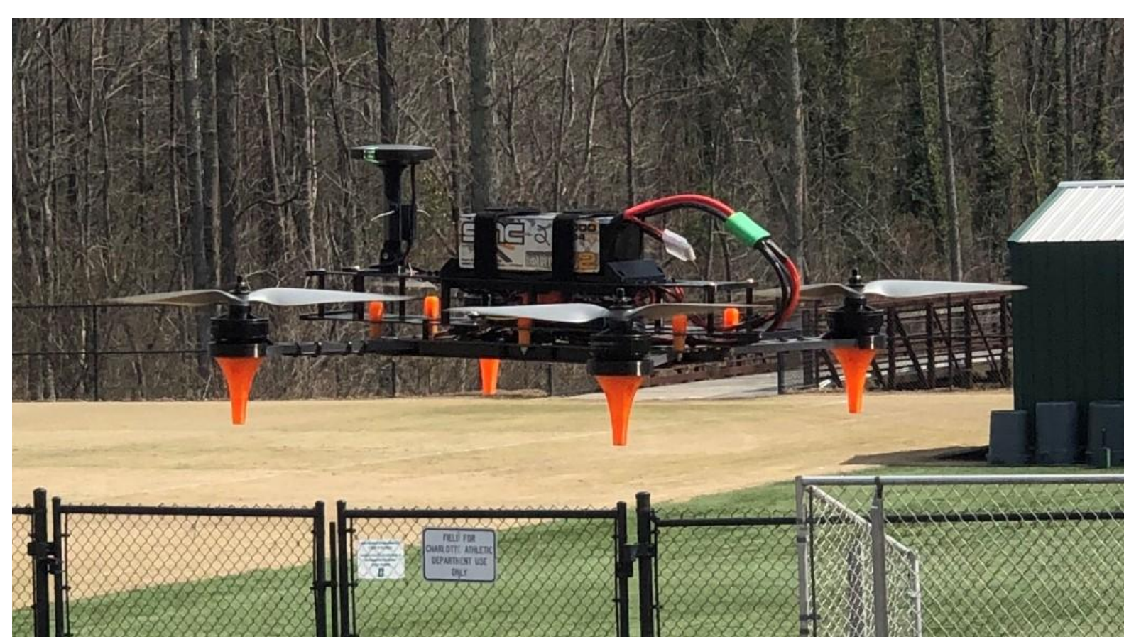
The custom-built quadrotor used in the experiment utilizes four Cobra CM-4008 motors with 11" two-bladed propellers.
